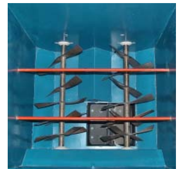
Dual Agitators Designed for Constant Flow
