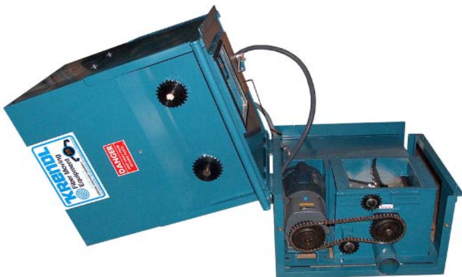
Airlock System 10" x 12" Diameter (25.4 cm. x 30.5 cm. diameter) 3" (7.6cm.) Outlet
